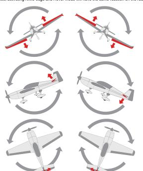
When the plane is rotated left or right (Roll). ailerons should have the correcting actions as illustrated above
